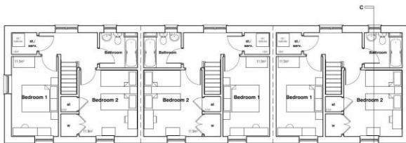
First Floor Plan
